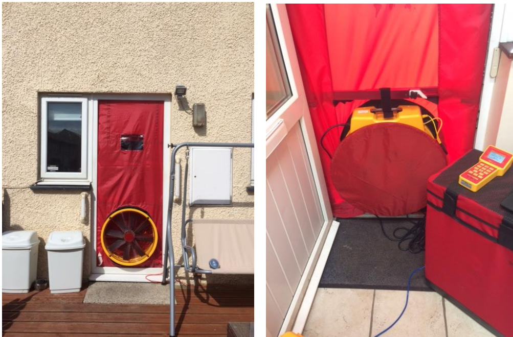
Figure 3.1 Airtightness testing of a property
