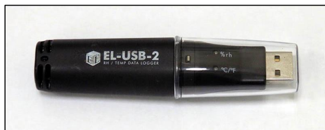
Figure 3.6 Lascar EL-USB-2 temperature and humidity logger
