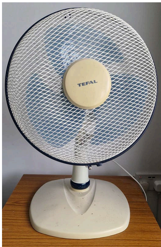
Figure 2.28 Tefal 14-inch fan rated at 45W
