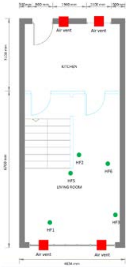
Figure 3.13 Schematic of heat flux sensors installed in property T-07 to measure u-value of the floor
