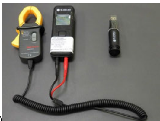
Figure 3.8 Lascar EL-USB-ACT current clamp Lascar EL-USB2 temperature and humidity logger
