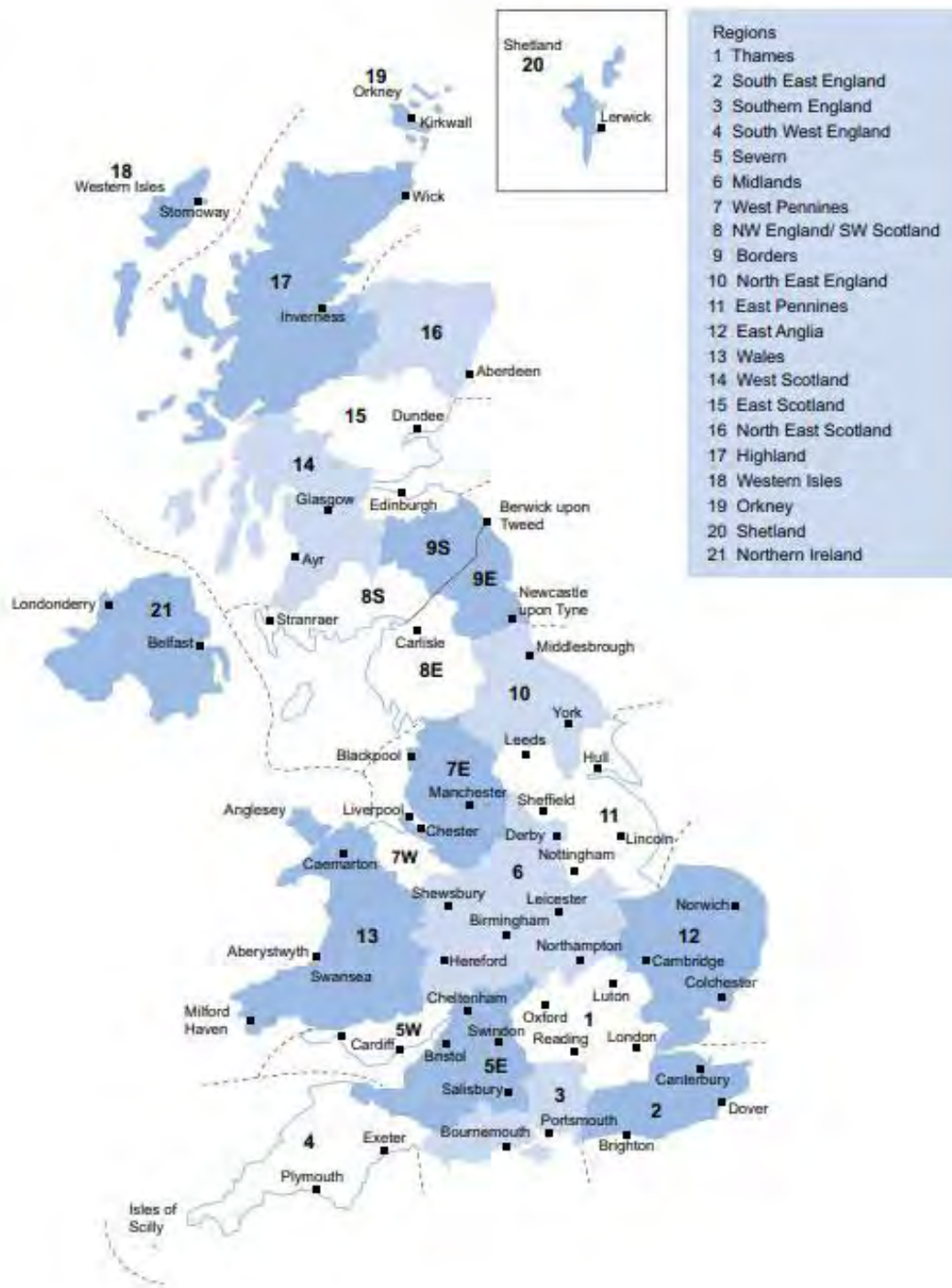
Figure 3.2 Map showing the 21 regions of the UK with tables for determining the value of Kk (From MCS MIS 3002 The Solar PV Standard) 3
