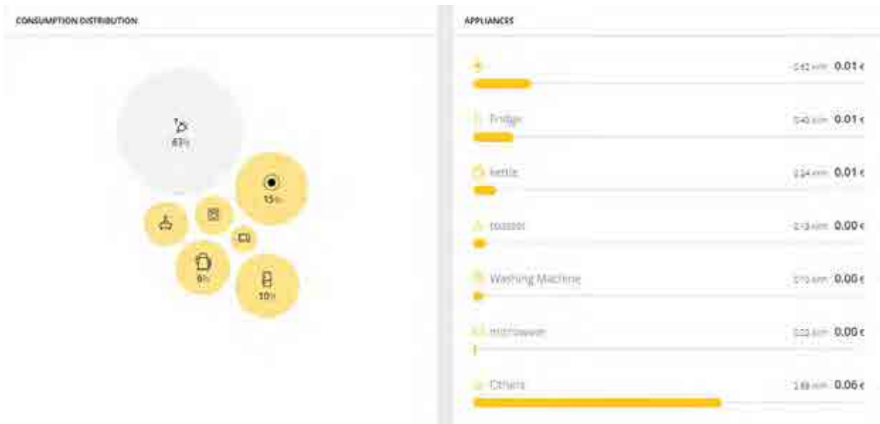
Figure 2.19 'Breakdown' section of Wibeer Nest portal showing disaggregation of the electricity consumption of different electrical appliances on 31 Jan 23
