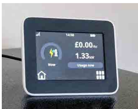
Figure 2.14 Chameleon IHD7 showing export of electricity to the grid
