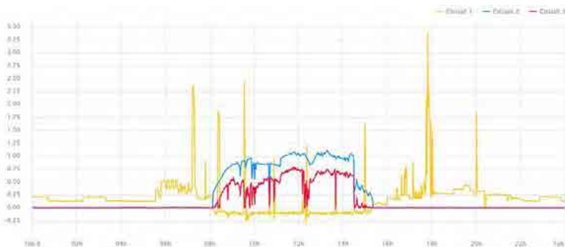
Figure 4.21 Plot of grid import/export (yellow) PV generation (blue) and consumption by the immersion heater (red) from the Wibeec Nest portal for household W-02 on 6 Feb 23
