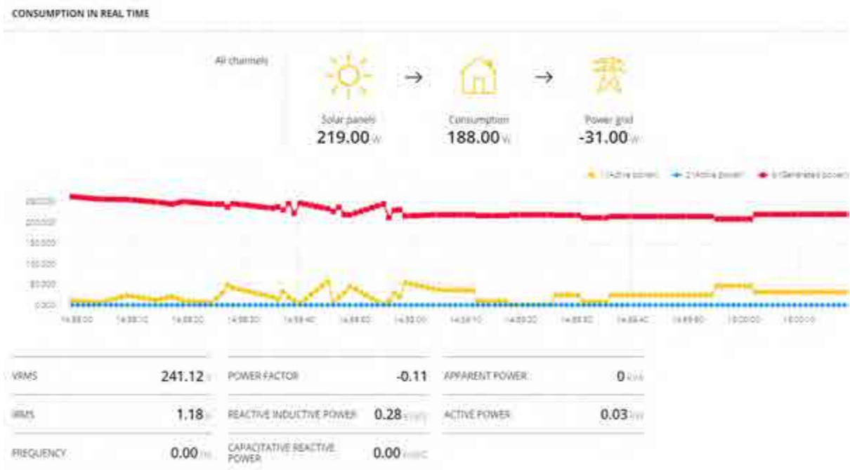
Figure 2.20 'Consumption in Real Time' graph from the 'Meters' section of the Wibeer Nest portal
