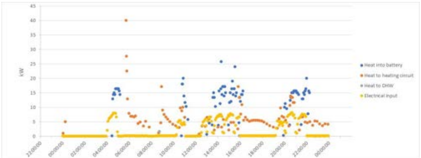
Graph 3.3.33 Property T-8 electrical input and heat outputs for 26 Jan 2017
