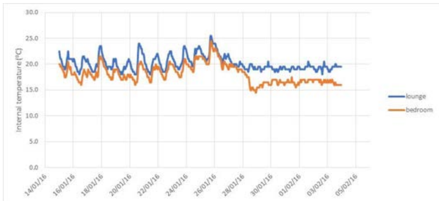
Graph 3.3.1 Property T-10 internal temperatures 15 Jan 16 to 4 Feb 16
