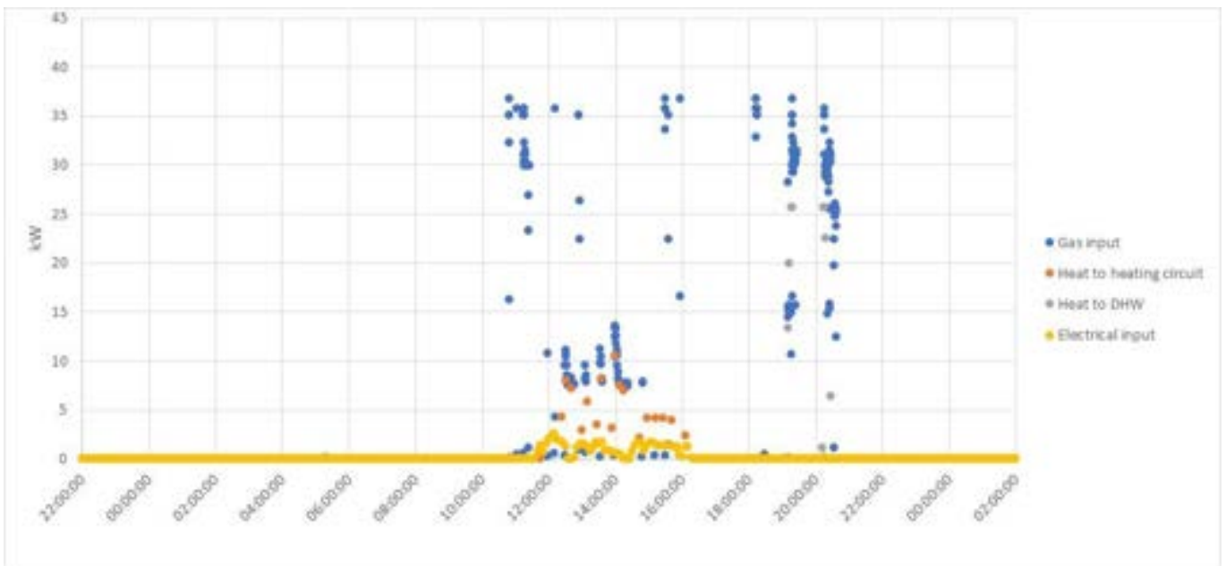
Graph 3.3.15 Property T-73 gas and electrical input to hybrid and heat output for 31 Jan 2018
