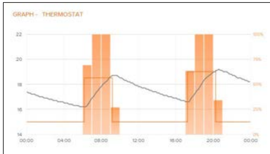
Figure 2.10 Graph plotted from the Netatmo web portal for a day in February, showing the actual temperature (°C, black line), set point temperature (°C, orange line) and boiler operation time (% , orange bars)
