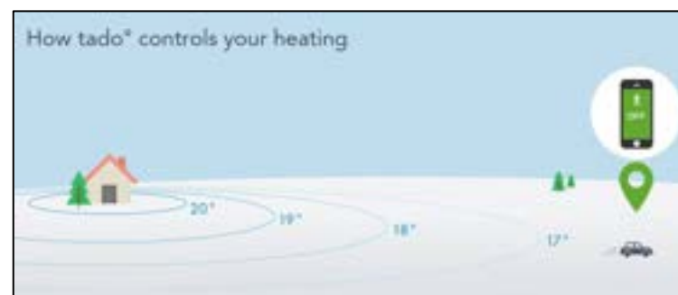
Figure 2.13 Diagram illustrating how tado turns down the temperature as householders leave the property.
