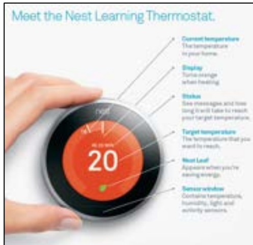
Figure 2.6 Nest smart thermostat controller
