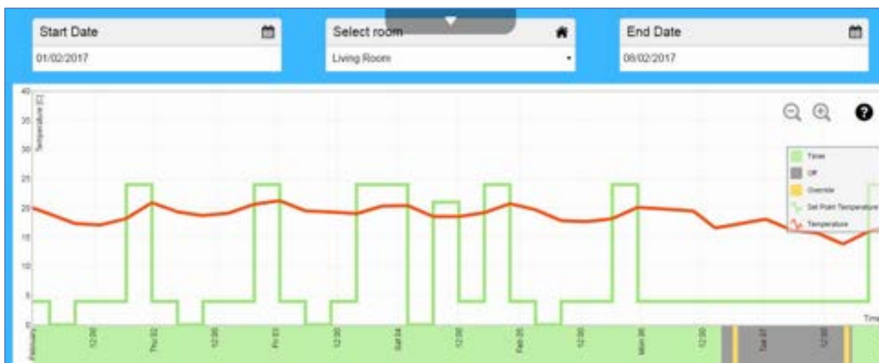
Figure 2.12 Historical temperatures and settings from the Heat Genius web portal
