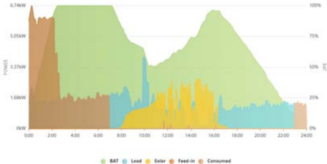
Figure 2.2 Power Diagram from the Alpha ESS battery portal for Household B-05 on 12 Feb 2024 with an Economy 7 tariff
