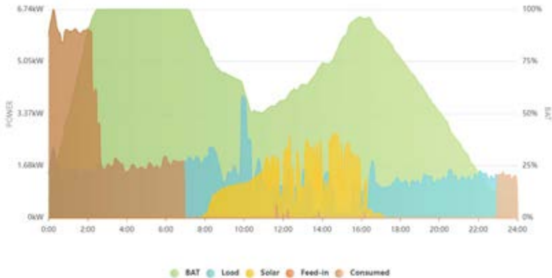
Figure ES3 Power Diagram from the Alpha ESS battery portal for Household B-05 on 12 Feb 2024 with an Economy 7 tariff
