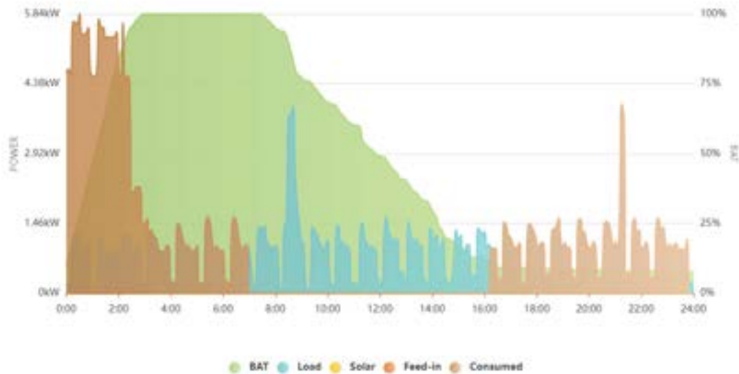
Figure 1.4 Power Diagram from the Alpha ESS battery portal for Household B-05 on 21 Feb 2023 with an Economy 7 tariff
