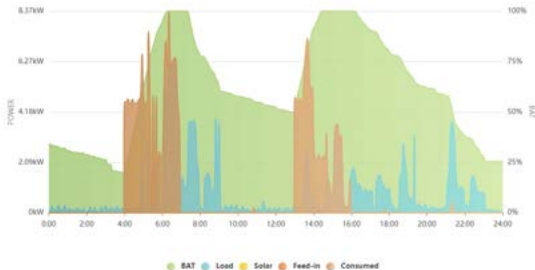
Figure 1.5 Power Diagram from the Alpha ESS battery portal for Household B-02 on 21 Feb 2023 with the Cosy Octopus heat pump tariff
