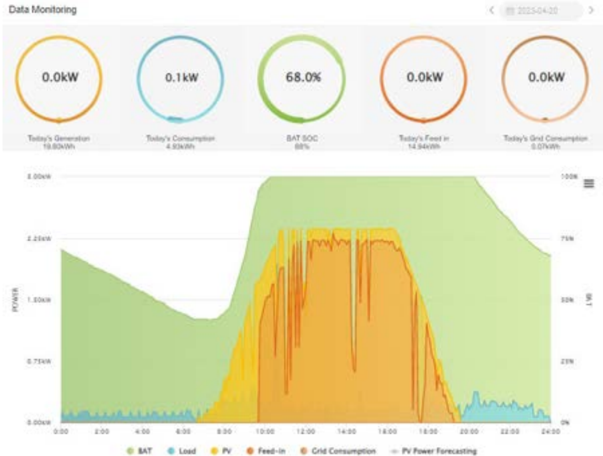
Figure 3.7 Power Diagram from the Alpha Cloud portal for an installation on 20 April 2023
