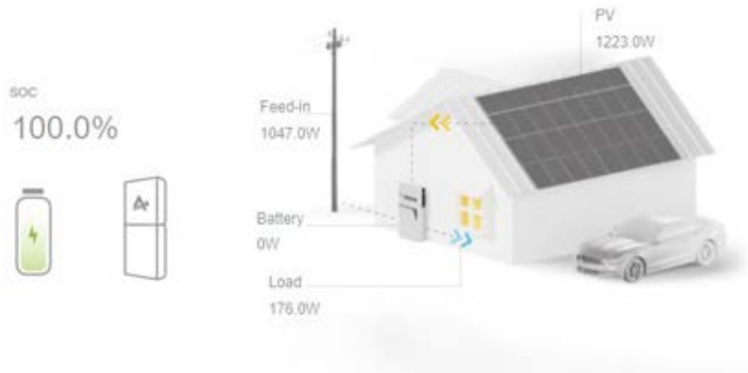
Figure 3.5 Real-time Power Graph from the Alpha Cloud portal on 19 May 2023 for a SMILE-B3 battery installed in the Smart Solar in Barnsley project
