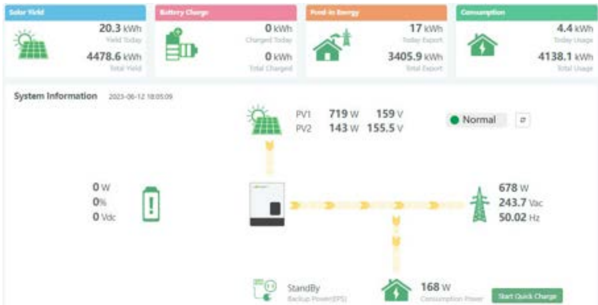
Figure E2 Summary and current system information from Monitor section of LuxPower portal
